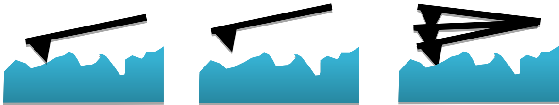
Figure 5: Working modes of AFM: contact, non-contact and tapping mode, from left to right
